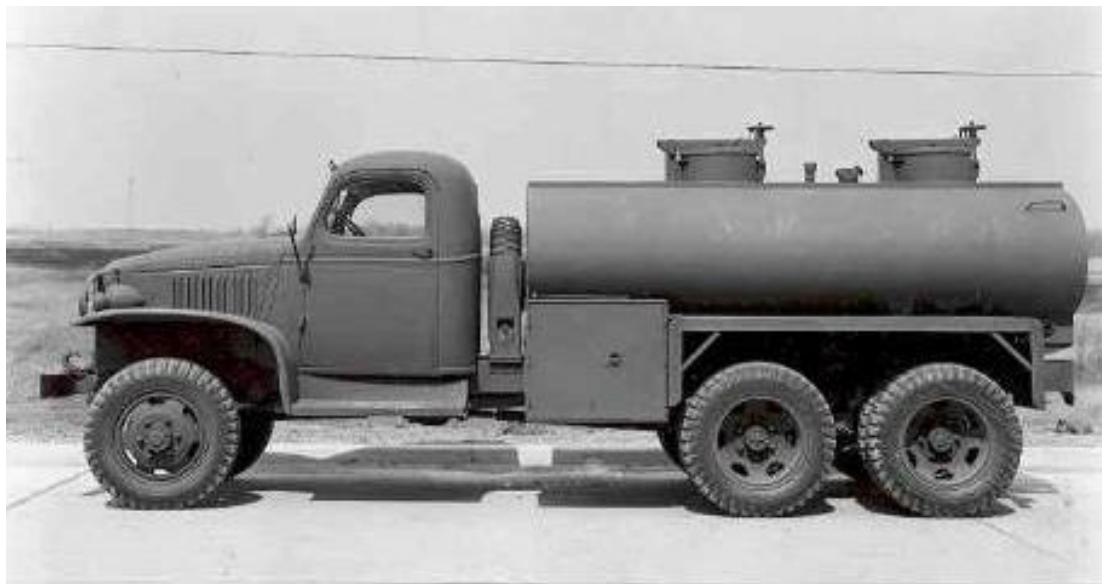
Afb. 10: Vrachtauto, tank: water, 2 1/2 ton, 6x6, 4DL. [Foto Internet].
