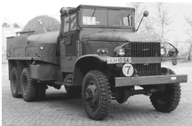
Afb. 5: Vrachtauto, Tank, Benzine, 2-1/2 ton, 6x6, 4 DL, LWB, GMC, Open cabine, z/lier. [Foto Museum Regimentsverzameling Technische Troepen]
