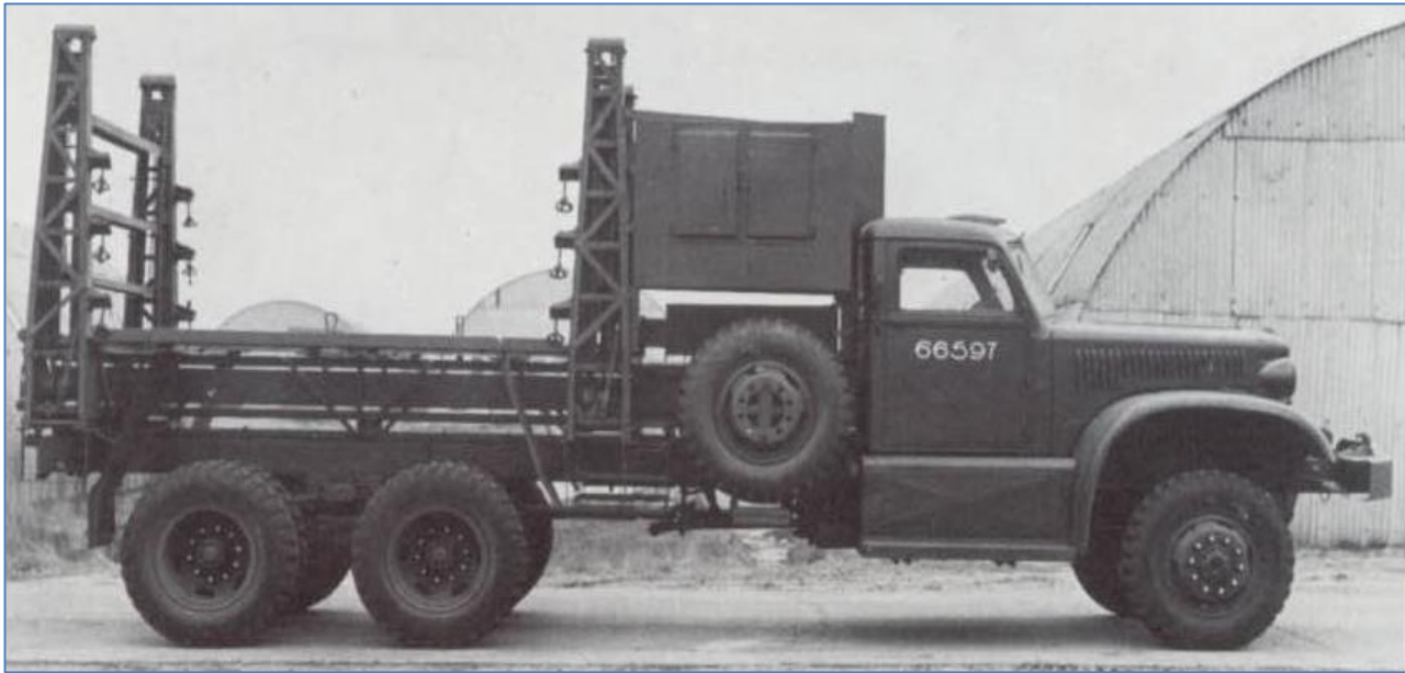
Afb. 7: Vouwbootauto, Diamond T, 4 ton, 6x6, 4dl, LWB, m/lier. (Lorry, 4 ton, 6-WH, F.B.E. (Folding boat equipment) 6x6, 201 wb.).
