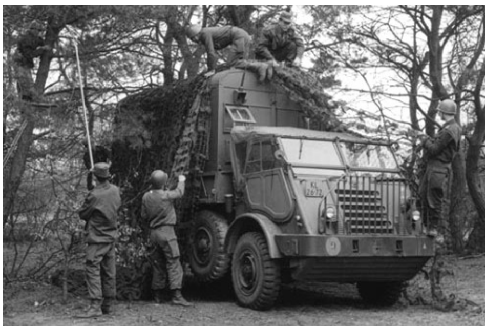
Afb. 4: Vrachtauto, Radio : 3 ton, 6x6, YA 328, m/shelter type HO-17-A.
