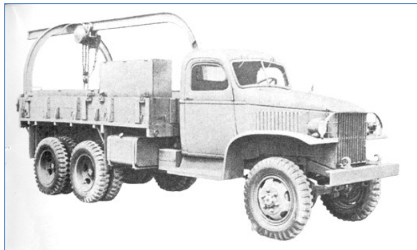
Afb. 7: Auto, Vracht : 2 1/2 ton, 6x6, 4DL, 6 V, LWB (164 inch), CCKW-353, m/monorail en takel, v/gasdienst, M1, (GMC).
